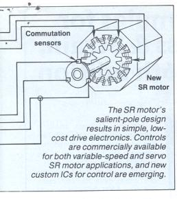
flux density, seeking an unsaturated portion of the circuit. The result is some sharing of back iron. To alleviate this problem, the unused segments of back iron between the phase pole pairs are simply removed.
