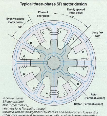
the back iron cause significant hysteresis and eddy-current losses. But SR motors, in general, have many benefits, such as low manufacturing cost, high speed, low inertia, low-copper loss, rugged design, and excellent heat dissipation.
