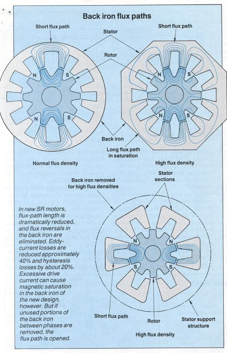
losses in the stator and in the rotor back iron. Also in conventional designs, all portions of the back iron are affected. Despite newer laminated, magnetically permeable, steel stator and rotor construction, iron losses still are significant.
