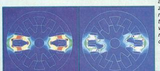
are aligned (left), zero flux and torque result. Maximum torque is produced with the stator and rotor poles offset (right). simply receive a series of pulses that advance the rotor a fixed number of degrees per pulse (1.8° for a 200-step motor), typically without regard to the rotor's absolute position. SR motors, on the other hand, are commutated like brushless dc motors — commutation depends on rotor position not clock pulses.
