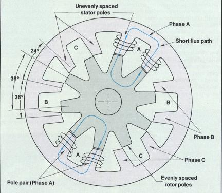
Pacific Scientific's SR motor excites poles in adjacent pairs to form a primary magnetic circuit. This substantially reduces the amount of back iron in the flux path and results in lower iron losses.
