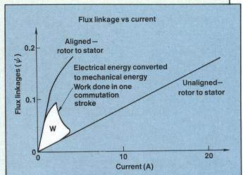
Continuous changes in air gap and pole permeance as the rotor turns, make the SR motors difficult to design. But new computer-aided design (CAD) tools are changing that scenario. Performance characteristics are generated in a dynamic computer simulation and displayed on the monitor as tables, curves, and geometric shapes. They help the designer fine tune the motor design and predict its behavior when installed in a system.
